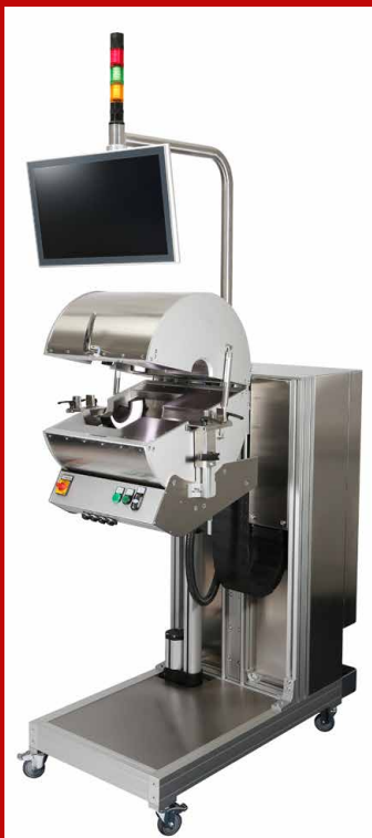
The sensor in the DualVision system ProfilControl 7 delivers surface information and dimensional data.
