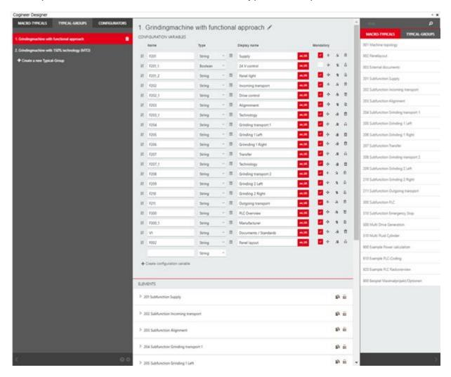
The third organizations structure in Cogineer Designer is formed by the socalled configurators. They consist of Macro-Typicals and / or Typical-Groups and are exactly the objects that are available in the Project Builder for the generation of schematics and partial circuits.
