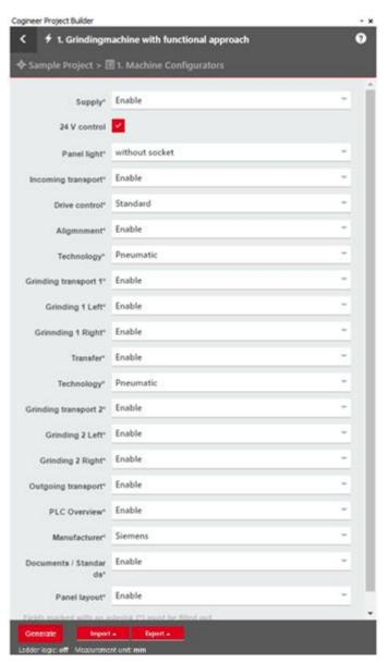
These configuration user interfaces are generated automatically and are always consistent with the definitions of the configuration variables in the respective Macro-Typicals or Typical-Groups. Changes in the configuration variables in Cogineer Designer are automatically visible immediately in the Cogineer Project Builder without special programming or another action of the user being required.
